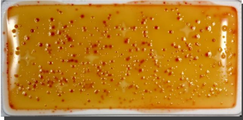
Example: Inoculated NUT/TTC paddle showing approximately 1000 CFU/100 mL.
